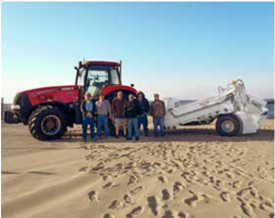
The beach cleaning team in Ocean City, Maryland, in front of their new BeachTech 2800 in the typical Ocean City look. The city purchased their BeachTech 2800 together with a “high tech tractor” and had the beach cleaner fitted with a direct drive for this tractor, so that they don’t need any hydraulic tank or cooler at the BeachTech. Contact us for more detailed information!
