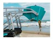
**© Collecting tank**The compact collecting tank has a loading volume of 0.5 m³.
