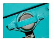
Maintenance-free bearings without lubricating nipples No need for regular re-lubrication.
