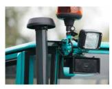
The BeachTech Marina is equipped with all safety features (acoustic warning alarms in the event of incorrect operations, reversing alarm, electrically operated exterior mirrors for optimum visibility,
