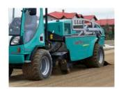
● Working width Working width of 1.40 m for coverage of up to 15,000 m²/h
