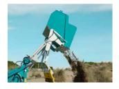
**© Collecting tank**The collecting tank has a loading volume of 1.5 m³.
