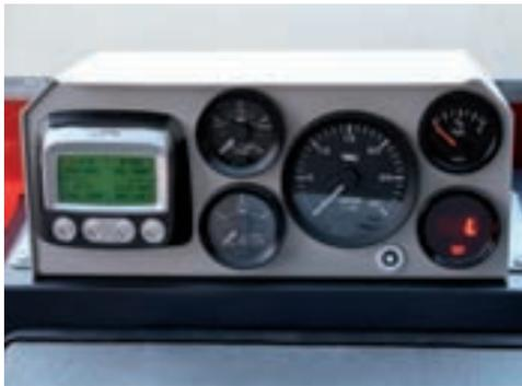
The display instruments on the PistenBully *Scout* are arranged clearly. All important data is available at a glance. The new PowerView Display bundles all information and can be programmed so that the engine switches itself off if preset values are exceeded. For example, this avoids a high revolution speed.
