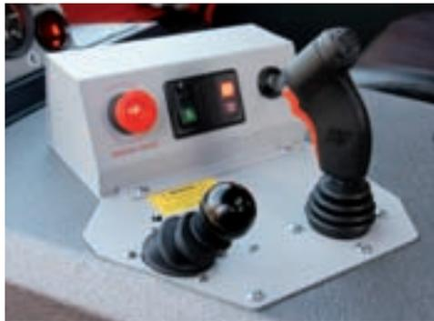
The electronic hand throttle is infinitely adjustable by lever. There are no disruptive cables in the interior.
