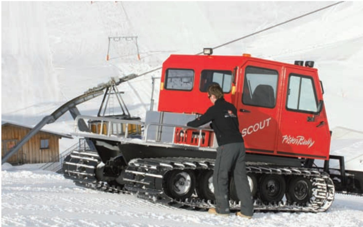
The PistonBully *Scout* platform is as flexible as its area of use is diverse. As a platform for transporting goods it offers enough space and reduces the number of trips required. Work material and tools can also be stored safely.
