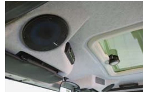
A successful combination of modern design and optimised functionality: the cloth headliner with improved thermal and acoustic insulation.
