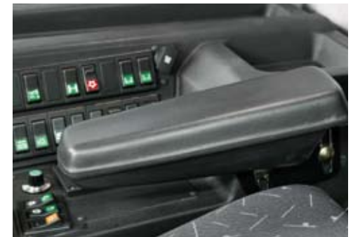
The armrest supports the driver's arm for fatigue-free operation of the front- and rear-mounted auxiliary attachments.
