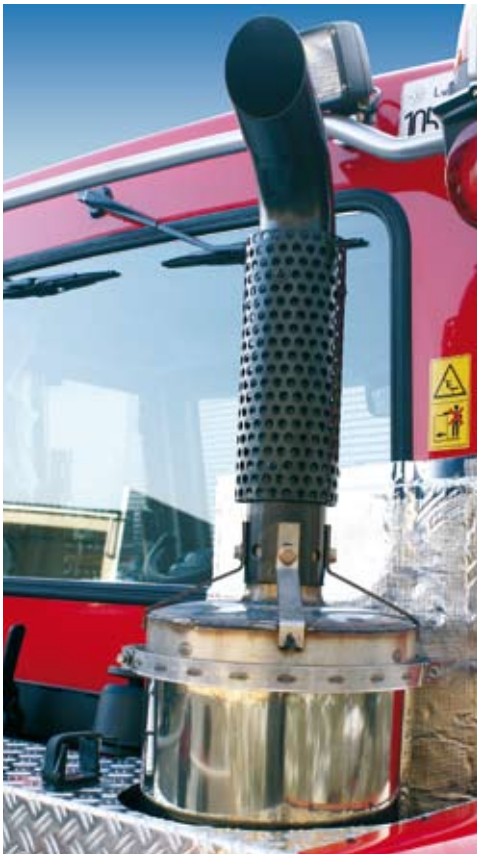
Integrated exhaust filter system and soot filter.
