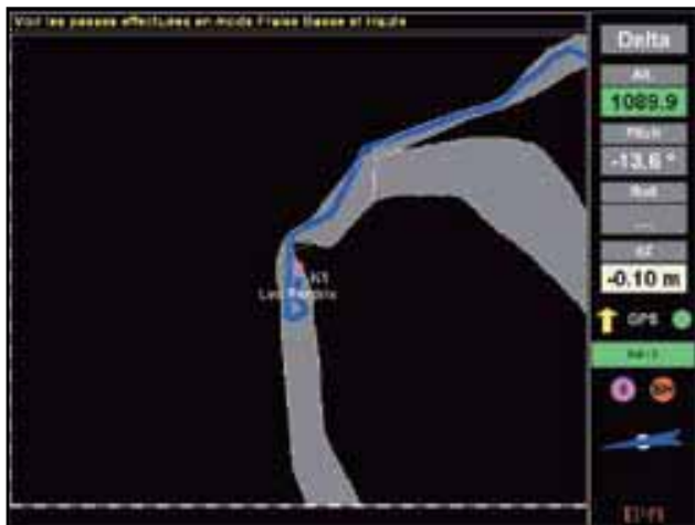
Cartographic image of snow depths in the cockpit with SNOWsat Package 4.
